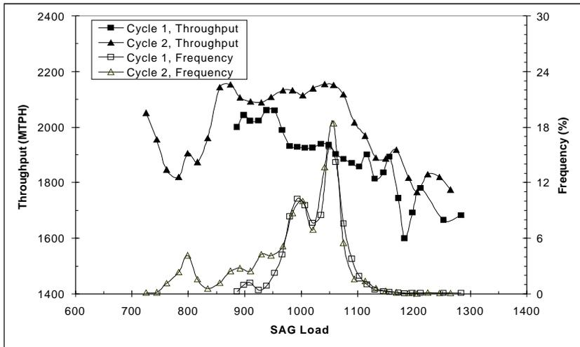
**Figure 2: Throughput Versus SAG Mill Load**
