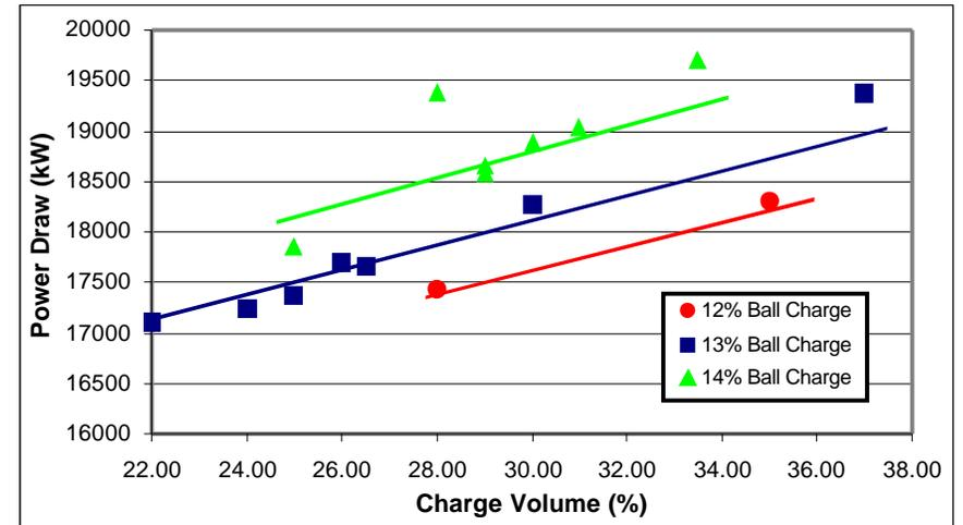
**Figure 3: SAG Mill Power Draw versus Load**
