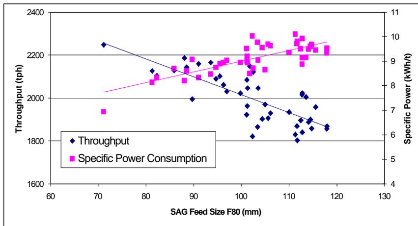
Figure 9: SAG Mill Feed Size Versus Throughput
