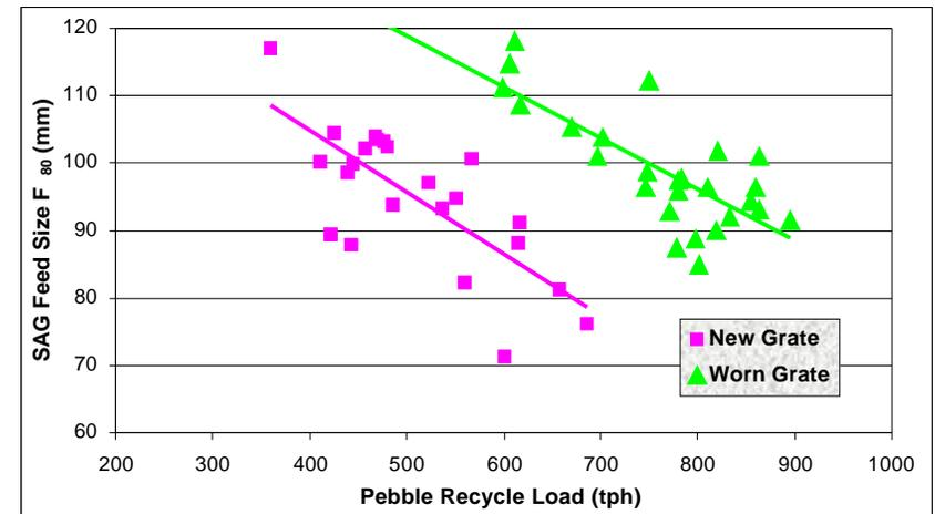
Figure 5: Comparison of Grate Performance (New/Worn) with Feed Size
