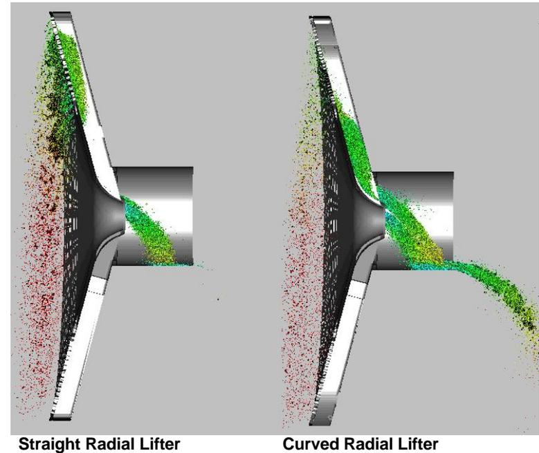
**Figure 7: Comparison of discharge rates from straight radial and curved pulp lifters.**
